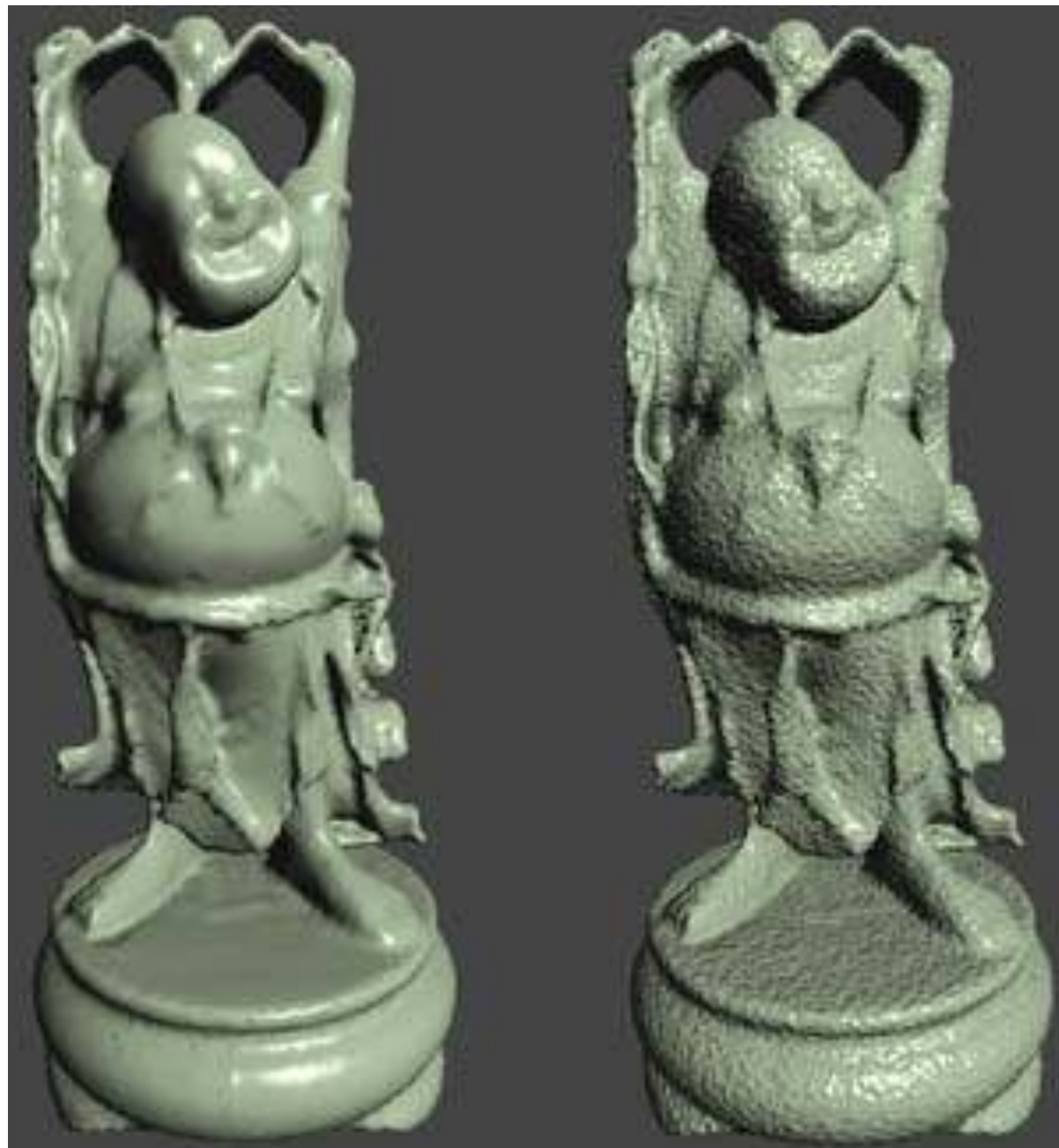
Procedural bump mapping, done by computing noise in the pixel shader and using that for perturbing the surface normal
