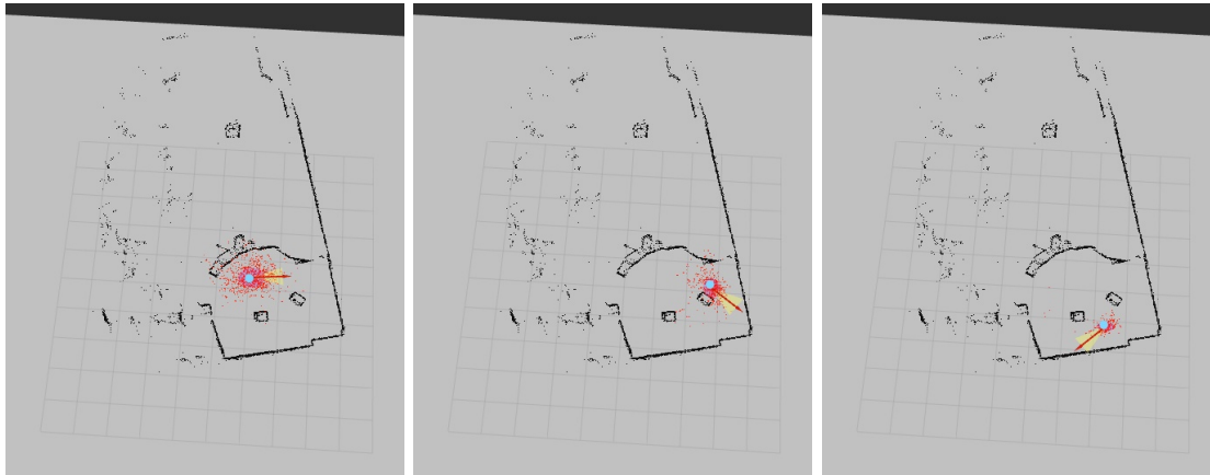
Figure 6: Convolution after Kidnapping with pose estimation (The blue dot is the actual robot position)
