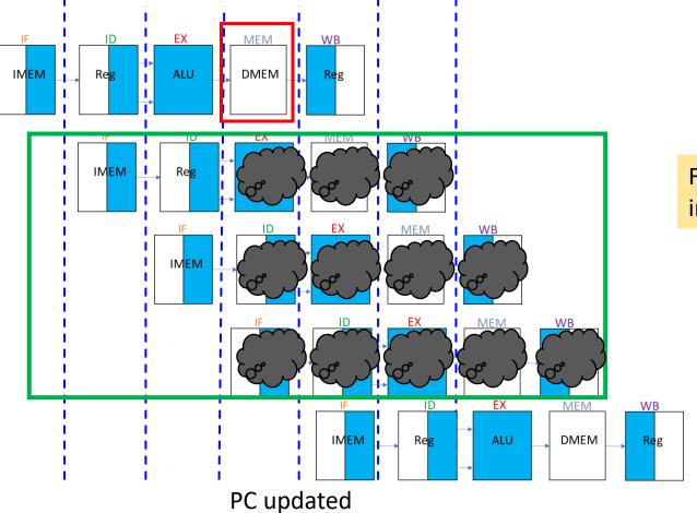
Flush pipeline by converting incorrect instructions to nops
