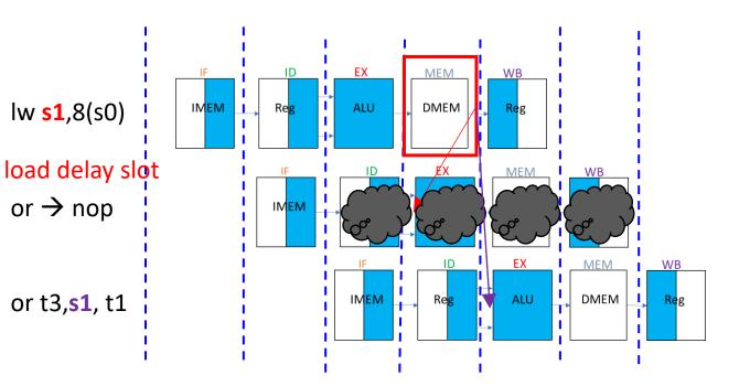
MEM stage (lw)'s output needed as EX stage (or)'s input in the same clock cycle.
