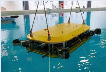
Cuttlefish — AUV with 2 arms
