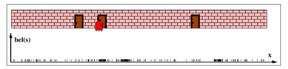
**Resample** the particle set based on weights, then **motion update** (apply noisy motion transformation to each particle).
