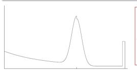
$$P(z \mid x, m) = \begin{pmatrix} \alpha_{\text{hit}} \\ \alpha_{\text{unexp}} \\ \alpha_{\text{max}} \\ \alpha_{\text{rand}} \end{pmatrix}^{T} \begin{pmatrix} P_{\text{hit}}(z \mid x, m) \\ P_{\text{unexp}}(z \mid x, m) \\ P_{\text{max}}(z \mid x, m) \\ P_{\text{rand}}(z \mid x, m) \end{pmatrix}$$
