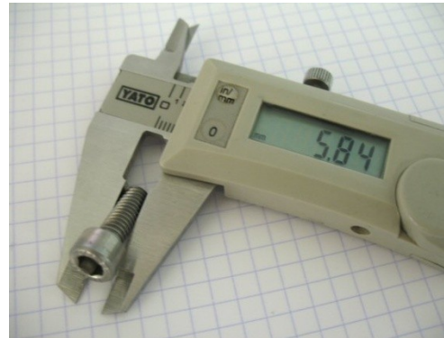
Outside diameter of M6 thread
