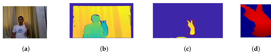
Figure 2. Simulation result of preprocessing step on HUST-ASL dataset: (a) Color image of the RGB-D images. (b) Depth map of the corresponding color image. (c) Localization of hand from the depth map using depth thresholding and removal of noise. (d) Resize of the hand segmented image according to pre-trained CNN input size.
